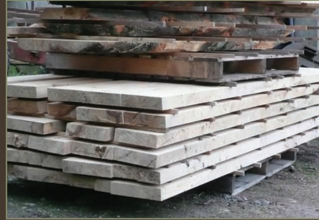
Sawn Timber prepared for Air Drying.
