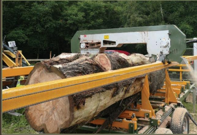
The Mobile Bandsaw Mill in action.
