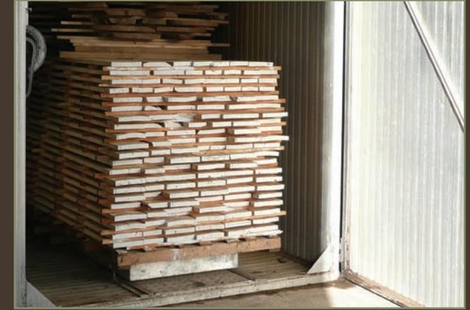
Kiln Drying the timber stack.
